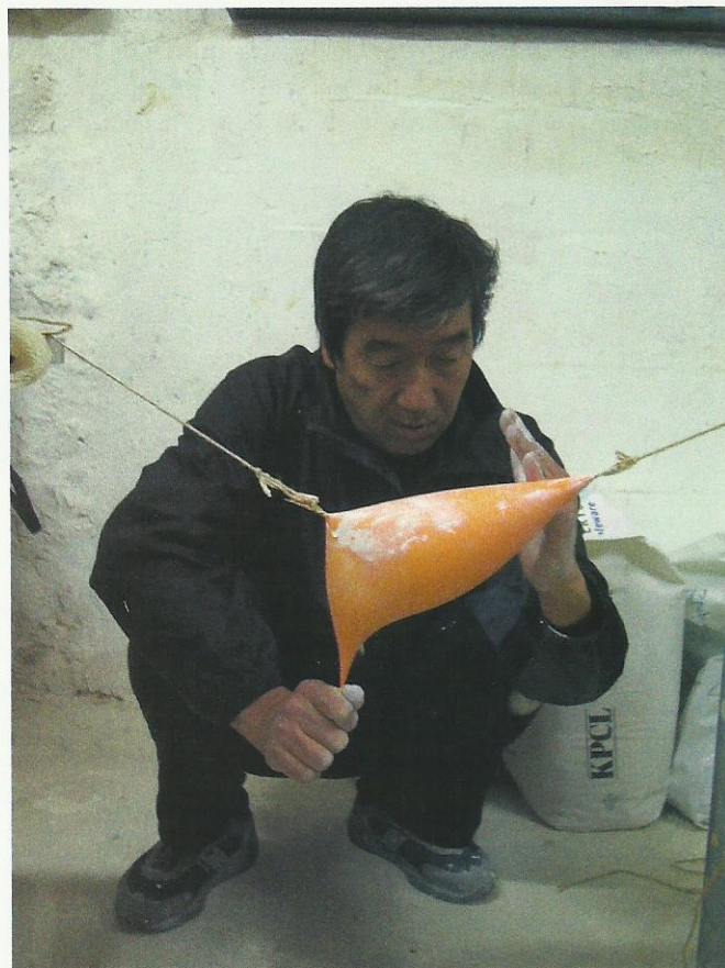
Hiroshi Itabashi demonstrating during his workshop, “Making Molds from Air and Water.” He fills a balloon with liquid plaster to make various shapes (here he makes the body of a pitcher). After the plaster sets, he makes a mold of the shape.
