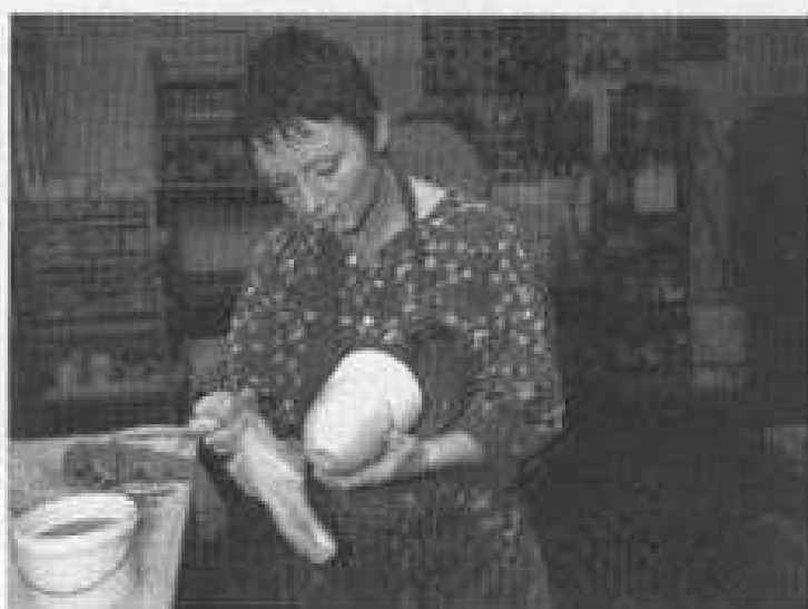
Figure 4. After the form has dried from applying the glaze on the inside, Patty immerses the pot in terra sigillata up to the glaze rim. When the terra sigillata is almost dry, the piece is burnished with a plastic shopping bag wrapped around her finger. Once dried, the pots are bisque fired to 2012°F (1100°C).
